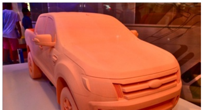
A resin-based prototype made with 3D printer.
