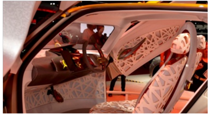
The internal structure of concept car made of fiberglass and nanotubes.
