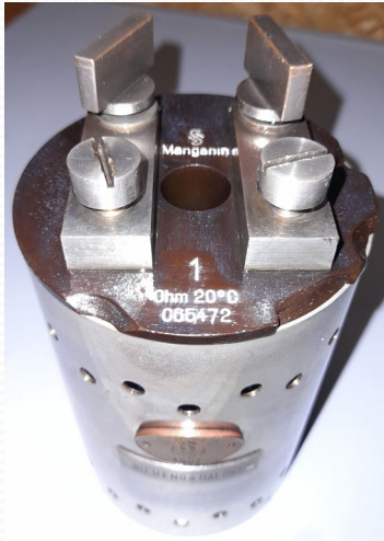
Resistor 1 \Omega (1907) (UTE)
